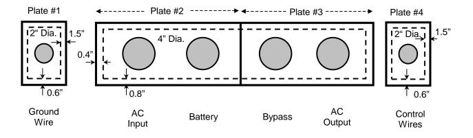
Four solid rectangles show the cable knockout plates' outline. The 3 dashed rectangles show the UPS opening under the plates.
